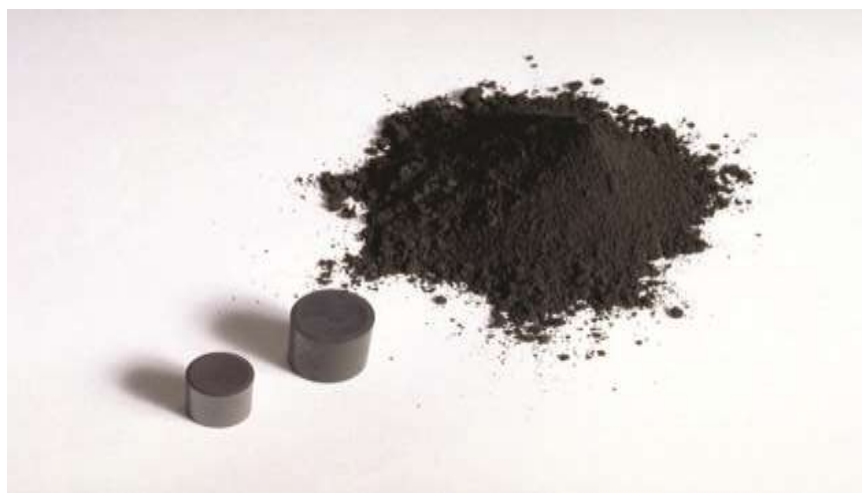
Uranium dioxide in powder and pellet form (CANDU)
