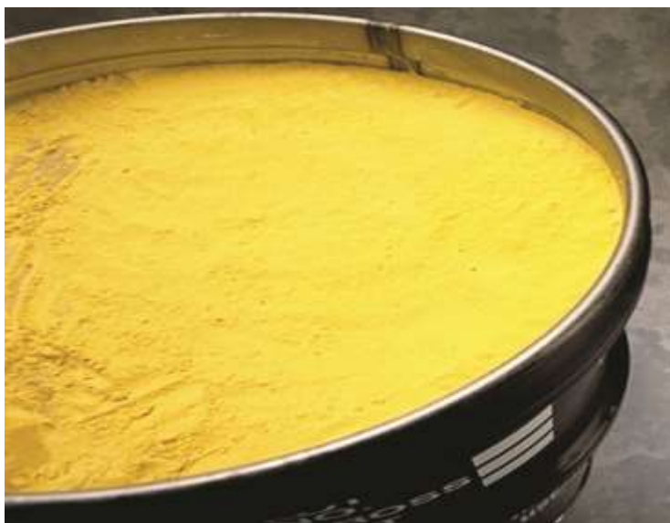
Yellowcake in a drum for storage or transport (Cameco)
